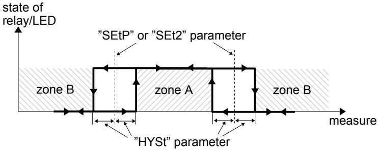
Figure 6.6. Two threshold control of the relay/LED outputs
