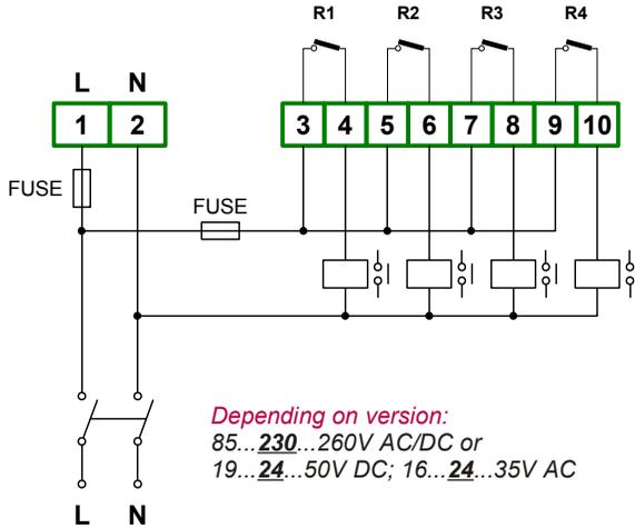
Figure 4.15. Connection of power supply and relays
