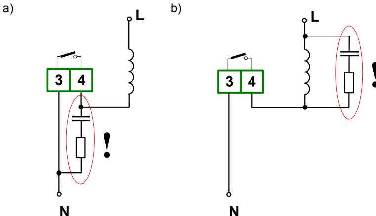
Figure 4.16. Examples of suppression circuit connection:
