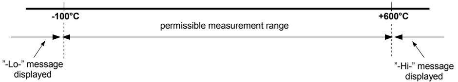
Figure 6.3. Definitions of measurement ranges in mode Pt100
