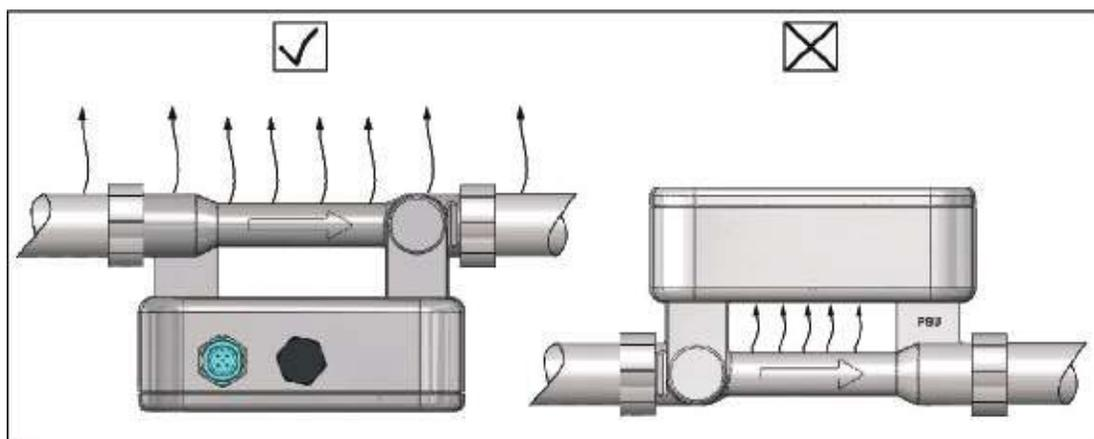
Fig. 6: UltraFlo with hot liquids
