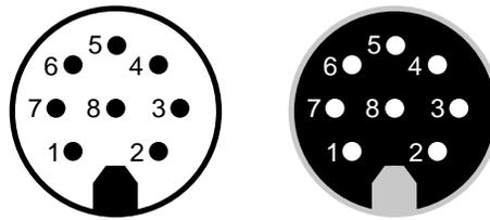
Fig. 8: Pin code: Connection plug / socket
