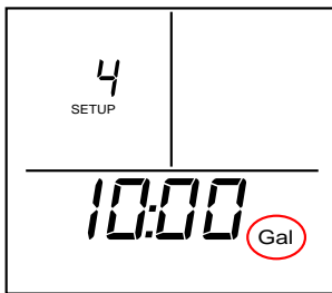
SETUP 4 – Programming the tank/drum/sump capacity (ltr./ Gal.) Enter the number in litres/ gallons then Press ENTER to save
